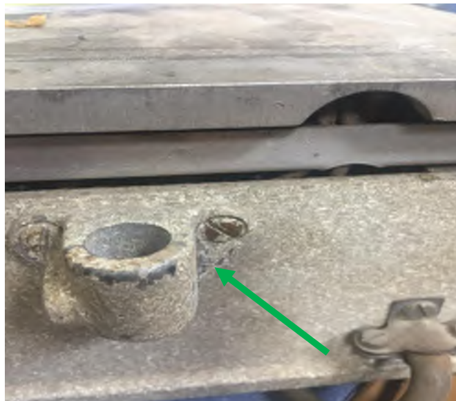
Photograph 2. Internal Insulation to hot plate, 27 Science, Science Wing; (FI0306). No asbestos detected.
