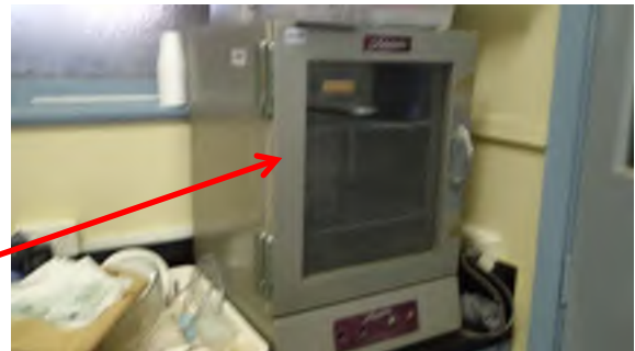
Photograph 42. Heat mats. 33 Science, Science Wing (DA7318). Asebstos Detected.
