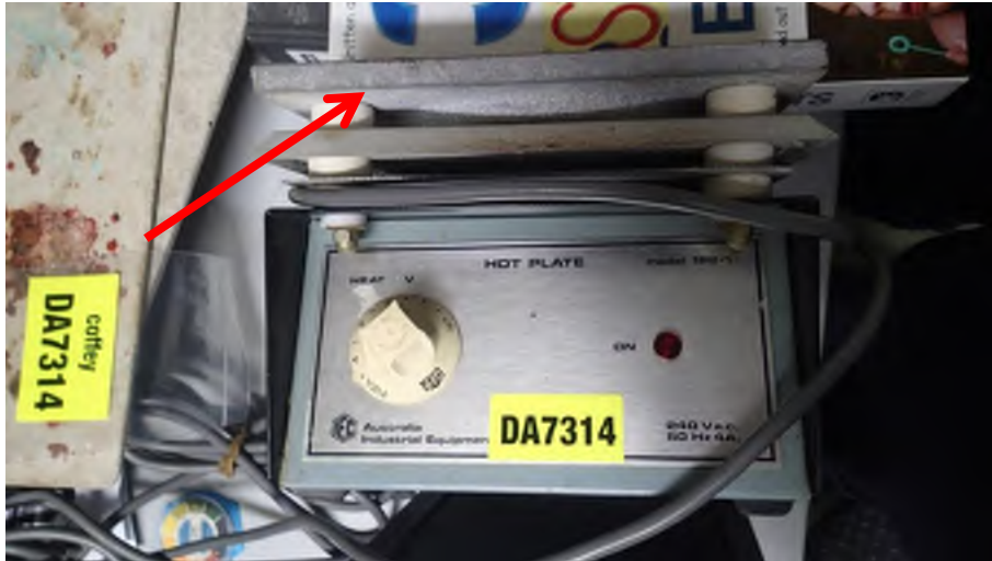
Photograph 1. Millboard lining to hotplate. 33 Science , Science Wing (DA7314). Asbestos detected.
