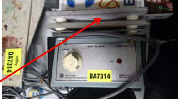
Photograph 43. Millboard lining to hotplate. 35 Store, Science Wing (Refer to 33538-39). Asbestos Detected.
